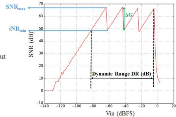
Overall gain of 90 dB (30 dB/stage) – 10-bit ADC
